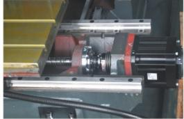
The three axes of T500 cobalt tapping center are all one-piece bearing pedestal, and all kinds of loads acting on the machine tool will eventually be transferred to the bed through various links, which greatly improves the dynamic performance and transmission rigidity of the machine. Due to some reasons such as processing difficulties and processing accuracy, very few domestic
