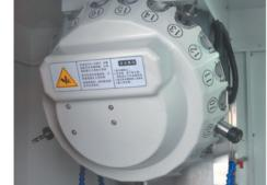
The special tool library in Jiangnan is designed with frequency conversion motor, which can be controlled by PLC software to achieve rapid tool change and more reliable performance. The cam drives the tool library to ensure the smooth operation of precision transmission when using heavy cutters.
